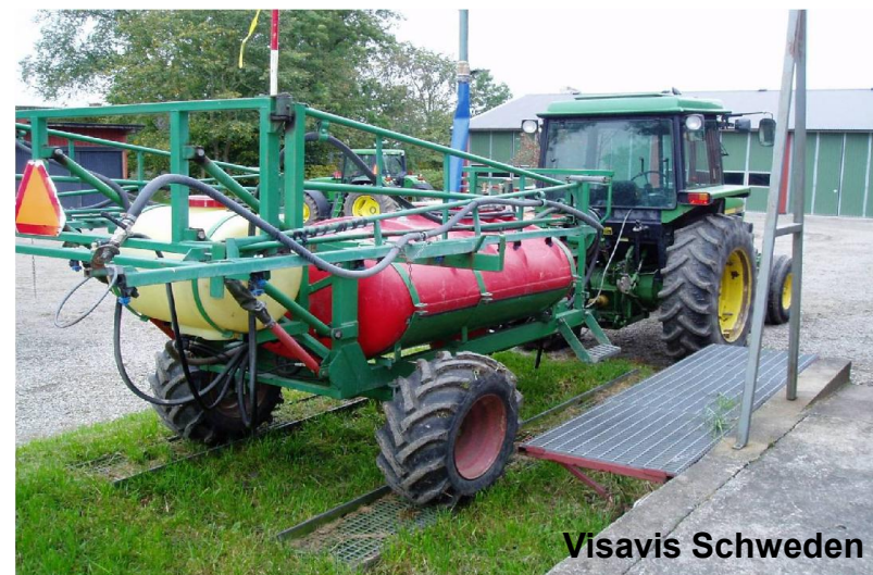
Filling place connected to slurry tank:LWK-NRW H.Kramer
