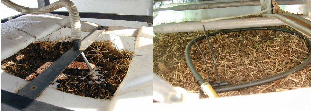
Fig. 21 & 22: Distributing the contaminated liquid over the surface by means of a metal plate (left, source CRAw) or a circular perforated hose (right, source pcfrit).
