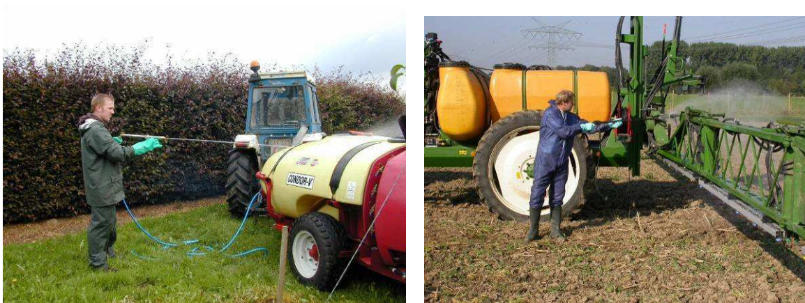
Fig. 8 & 9: cleaning the outside of an orchard/ tree crop sprayer (source: pcfuit) and a field crop sprayer (LWK-NRW)
