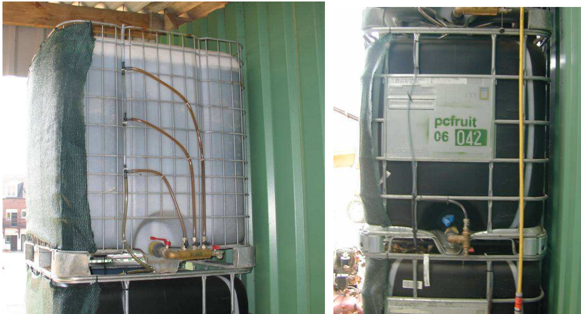
Fig. 35 and 36: To provide an optimal moist balance in 2 top units of the modified biofilter, a saturated zone is kept at the bottom of the unit to allow water to rise up through capillary force. This can be achieved by connecting the outlet of the unit to a pipe that is bend upwards and has an air duct leading to the top of the unit. The height of the saturated zone is determined by the height the outflow pipe is bend upwards. Different heights can be made (left) to choose from, or on saturated zone of 300 litres can be sufficient (right). After bending the outlet pipe, lead the end to the top of the next unit and distribute the leachate as shown in pictures 21-24. Other valves on the units in the pictures are used to sample the system, or to drain the system for winter storage and prevent the valves from freezing. (Source: pcfruit).
